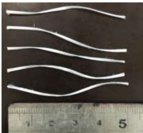
Figura 25 – Fibra TUF-STRAND-SF 51mm.
