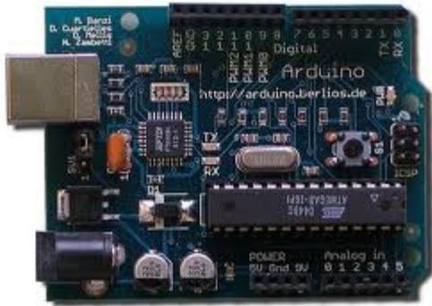
Figura 4 – Placa Arduino [10]
