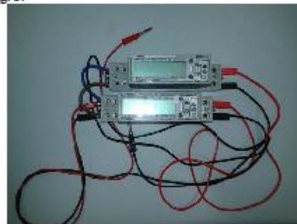
Fig. 2. Power network analyzer used in the experiments
