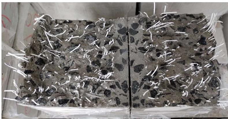
**Figura 45.** Seção transversal CP04 Concreto<sub>BFRP</sub>.
